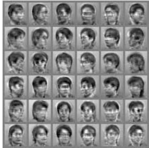
(a) The learned basis vectors. They are arranged according to the topology of 6 \times 6 torus lattice.
